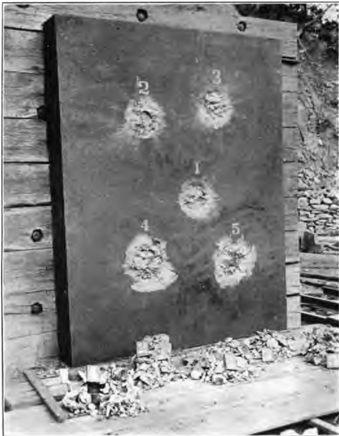
HARVEY ARMOR PLATE, TESTED NEAR BETHLEHEM, PA., JULY 30, 1892 104-inch Harveyed nickel-steel. Five shots from an 8-inch gun. Projectile, 250-pound Holtzer. Velocity, 1,700 feet per second.
